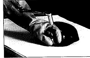
2. Then install the valve adaptor to a torque value of 90 in.lbs (10 Nm). (For the two piece valve stem design).
